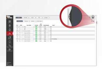
The logical view of the switch can be displayed on any NT5000 web page by simply clicking the <sup symbol located in the upper right corner of the page.
