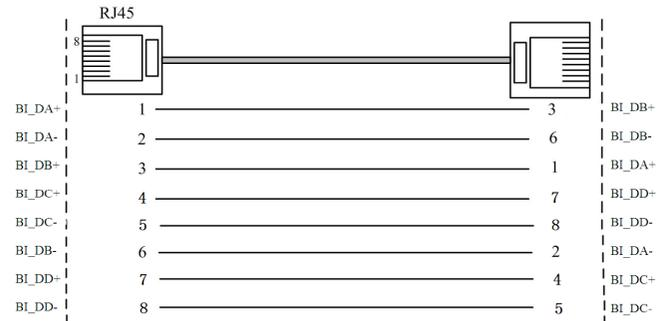
MDI/MDI-X auto connection makes switch easy to use for customers without considering the type of network cable.
