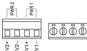
The switch top panel provided 4 bit power supply input terminal block, support DC input. DC power supply input supported redundancy function, provided PWR1 and PWR2 power input, can use for single, and can connect 2 separately power supply
