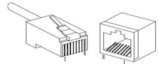
RJ 45 port support automatic MDI/MDI-X operation. That can connect the PC, Server, Converter and HUB. Pin 1, 2, 3, 4, 5, 6, 7,
