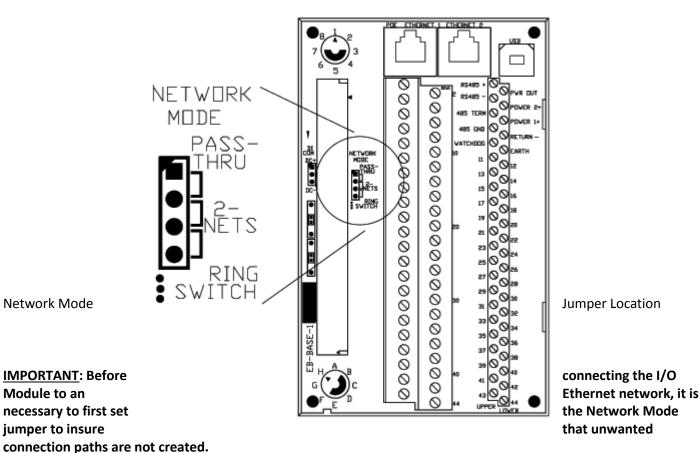
NOTE: The jumper is located on the base so that the replacement of a module or inadvertent change in configuration will not adversely affect the network.
