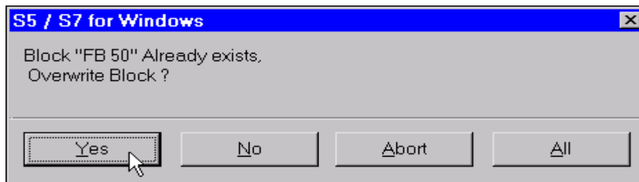
Figure 3-98 PLC Block already in PLC dialog box
