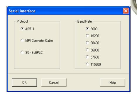
The Simatic S5 PLC must be connected to one of the serial ports (COM 1 – COM 4) of your PC via a 20mA current loop converter. Select the AS511 (Simatic-S5) protocol for the communication.
