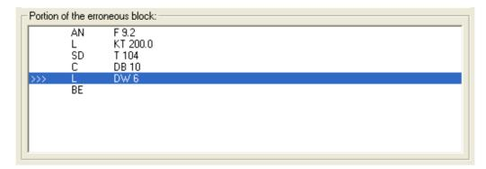
A pull down list field is provided to display the portion of the PLC where the fault occurred. The statement where the PLC went into a STOP condition is displayed with a blue background.
