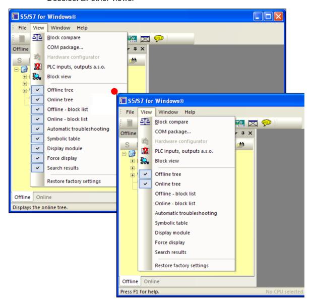
The "Offline tree" is used to select the "S5 Project" you want to work with. The S5 Project contains the files necessary for a S5 PLC program. Further on it will be explained how to generate a S5 Project. An S5 Project is always required to work with a S5 PLC program executed on a PLC.
