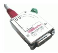
connection via a switch, a hub or even directly to a PC with a common network adaptor. The protocol used is the standard TCP/IP protocol. In this way, the user can benefit from all the advantages of Ethernet, such as remote maintenance via a standard router or VPN-connections (Virtual Private Network). Likewise, a direct connection to the Internet is possible.
