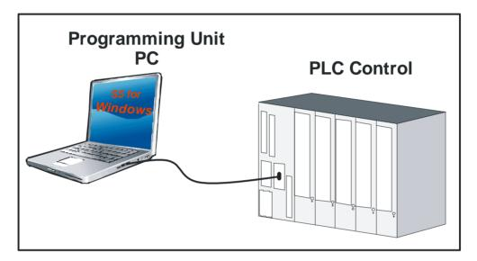
The S5 PLC's connected to the PC are listed in the "Online - Tree".
