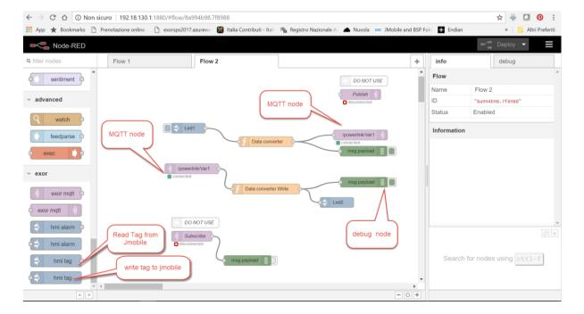
In order to connect to Amazon, Azure and IBM Bluemix we created specific exor Mqtt node with some predefined configuration parameter
