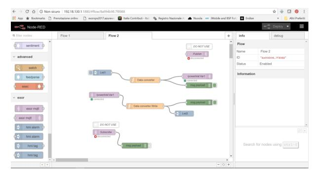
Led1 represets a variable called Led1 read from Jmobile runtime and sent to CloudMqtt free portal (<a href="https://www.cloudmqtt.com/">https://www.cloudmqtt.com/</a>)
