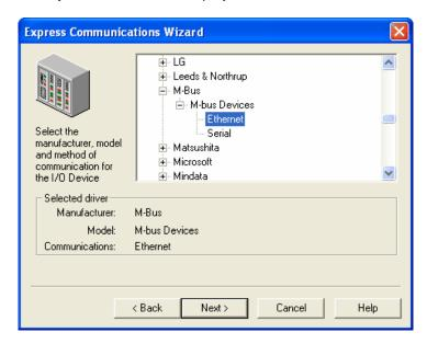
If you are using Ethernet communication we suggest you to use UDP depending of that M-Bus is a half duplex protocol and with UDP the driver will have full control if any faults as retries and timeouts should occur.
