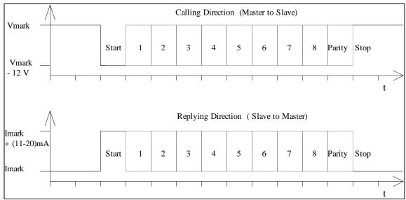
Transmission of a Character in Calling and Replying Direction
