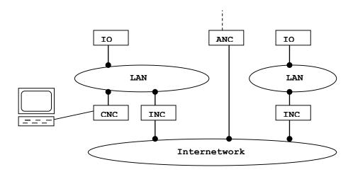
The CNC device is connected to a local Trend network (LAN) to which a number of devices (max 116) can be attached. Among those can be an internetwork device (INC) that links the local network to other Trend networks via an internetwork. To this network other networks can be linked via INC:s or ANC:s. The maximum number of devices on the internetwork is also 116.
