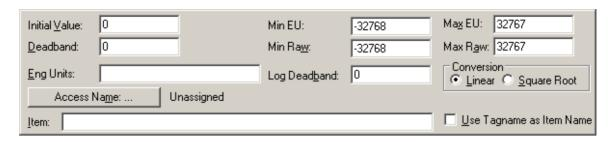
Select the Access name for OmronCIP Server by clicking on the **Access Name:...** button. The "Access Names" dialog box will appear:
