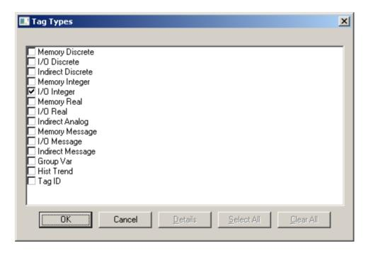
To access OmronCIP items, the type must be **I/O Discrete**, **I/O Integer**, **I/O real** or **I/O Message**. Select the Tag type.
