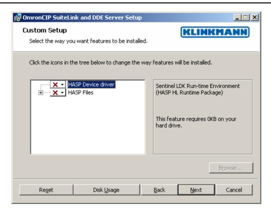
In case "HASP Device driver" and "HASP Files" **are selected** then HASP USB key will be supported and both HASP-key and software license will be available (files needed for HASP USB key will be installed):
