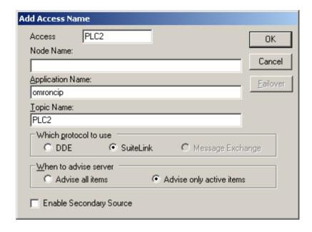
**Note:** If <u>Add</u> is selected, this dialog box will be blank when it initially appears. Data has been entered here to illustrate the entries that are made.
