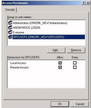
5. Now the configuration of OPC Server is completed – close the dcomcnfg program and restart the OmronCIP OPC Server to put new settings into effect.
