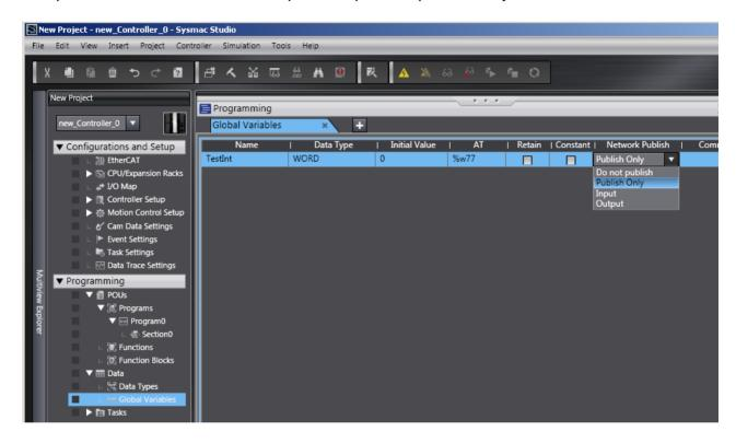
OmronCIP Server uses *Global Variables definition file* exported from Omron Sysmac Studio programming software to validate the corresponding Topic (Controller) item names and their properties.
