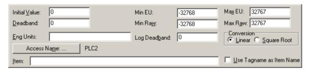
For integers and reals fill in the **Min EU**, **Max EU**, **Min Raw** and **Max Raw** fields. These fields control the range of values that will be accepted from the Server and how the values are scaled. If no scaling is desired, **Min EU** should be equal to **Min Raw** and **Max EU** equal to **Max Raw**.
