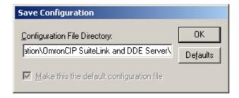
This dialog box displays the path where the Server is going to save the current configuration file. The path may be changed if necessary. Also, the path can optionally be recorded in the **WIN.INI** file by selecting the "Make this the default configuration file"
