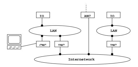
The CNC device is connected to a local Trend network (LAN) to which a number of devices (max 116) can be attached. Among those can be an internetwork device (INC) that links the local network to other Trend networks via an internetwork. To this network other networks can be linked via INC:s or ANC:s. The maximum number of devices on the internetwork is also 116.
