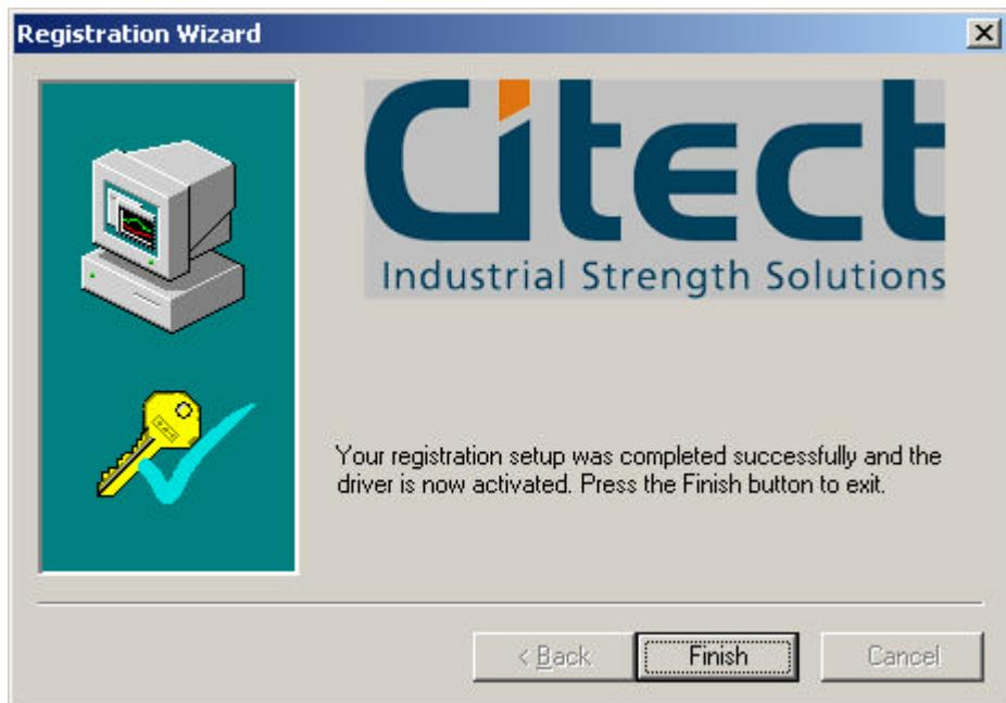
If you cancel the registration process, the 'Unregistered Driver' dialog box will remain open. If the 'Finish' button is pressed (process finished successfully), the dialog box will close automatically.
